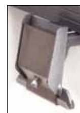
Fitting system for the rain gutter on the vehicle.
