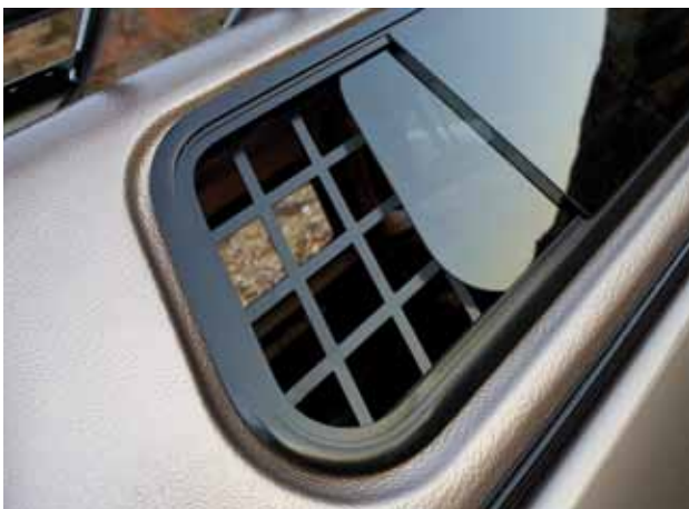
Side window safety grill
