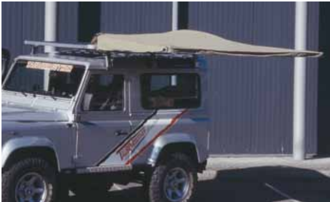
Special awning , no ground support needed size: 180 x 280 cm – only available for racks 200 cm long and over. Part-Nr.: 36-800977
