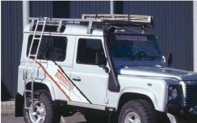
Foldable universal ladder , lays against the wheel. Easy access to your roof rack (roof tent) Part-Nr.: 36-800956
