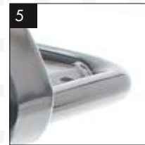
5 Rails are bent with a mandrel bender ensuring an even wall thickness across all sections
