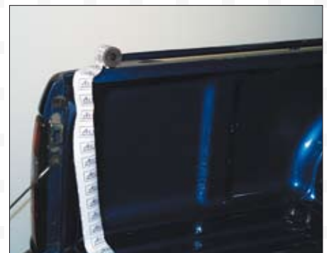
The liner tape gives superior protection from scratches in the rub zone between the liner and the vehicle paint.
