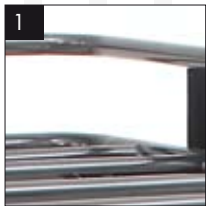
1 Top rail sits well above rack floor to ensure a secure load.
