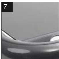
7 Air deflector plate significantly reduces wind noise.
