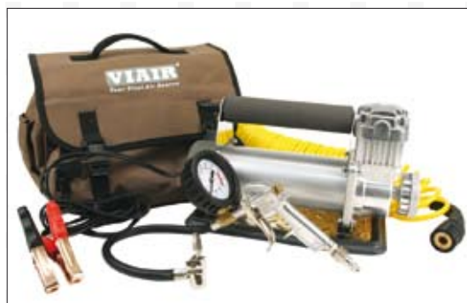
The VIAIR 450P-Automatic is the first portable compressor suitable for extended running. It can be operated at a pressure of up to 7 bar for hours on end without interruption. It has an automatic sitch-off function if no air is required. A simple push on the filling gun is all that is required to switch the compressor on again.
