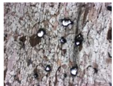
Copy snorkel material – distinctly grainy or crystal-like structure where additives and colouring agents simply coat the base material. Consistency varies markedly throughout.
