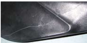
Impact damage – cracked snorkel body from a blow that barely marks the surface of a genuine Safari snorkel.
