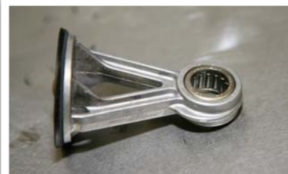
The ARB conrod utilises roller bearings instead of ball bearings to provide a superior rolling surface.
