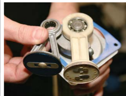
The ARB piston and conrod (left) is larger diameter and a shorter throw than others, which is one way of making the overall design smaller.
