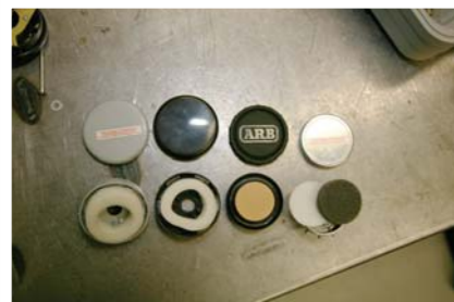
Air cleaners aren't all the same – the ARB sintered bronze unit (second from right) is designed to keep bull dust out and is washable. Some other's foam filters are a little suspect and couldn't be relied on.
