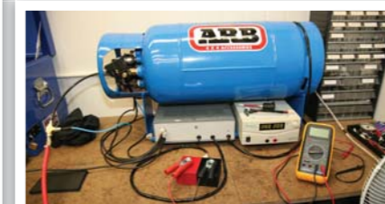
The ARB engineers designed and built their own compressor Dyno system to test and help build their own CKMP12.
